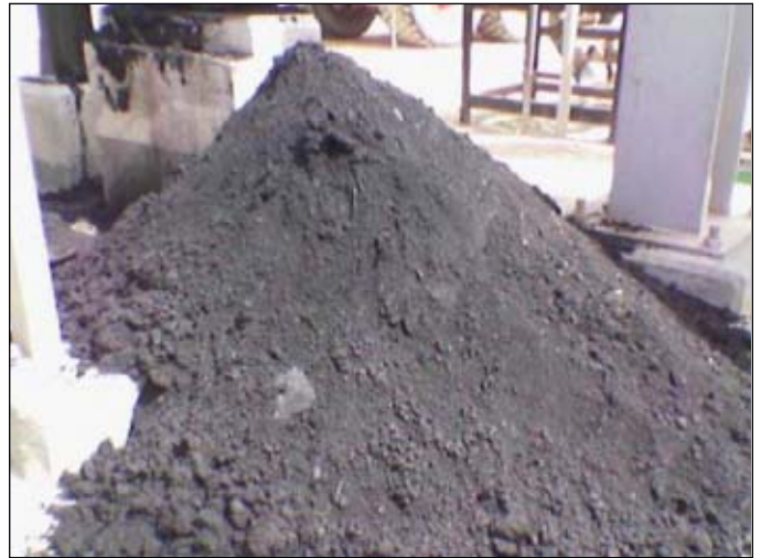
Black powder more often manifests itself as a dry, fine powder, as pictured here (Fig. 2).
